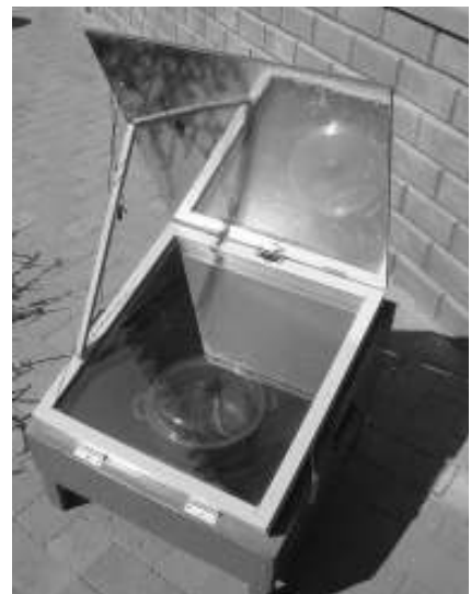
Solar box cookers reach temperatures of up to 150° (photo: Robert Schultz)
