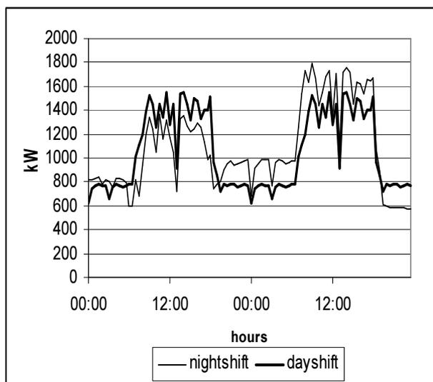
Figure 1: Typical dayshift and nightshift profiles during April 2005
