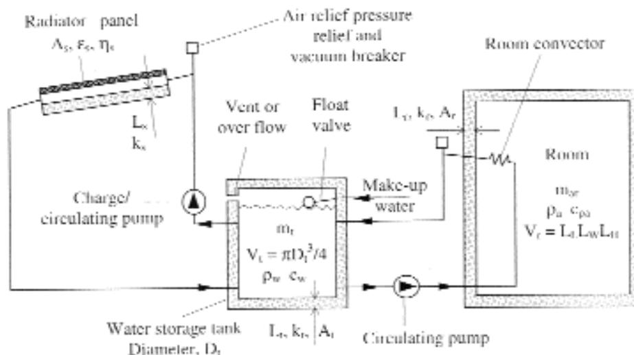
Figure 1: Thermal model of the night sky radiation cooling system showing the important components, variables and parameters
