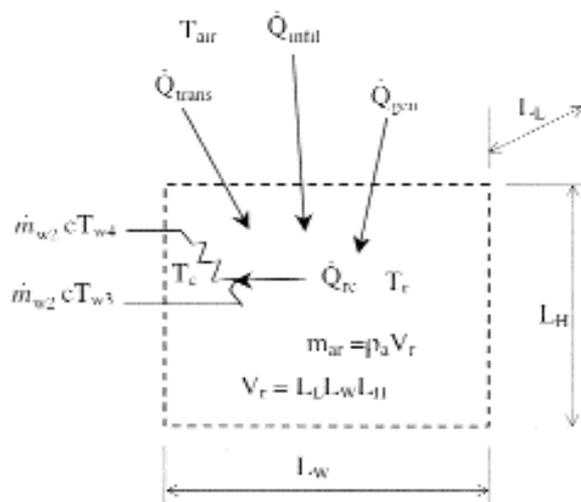
Figure 5: Room control volume including the convector
