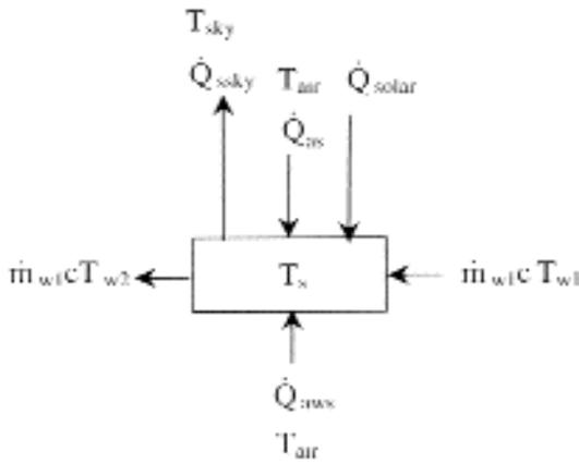
Figure 2: Control volume for the radiator panel
