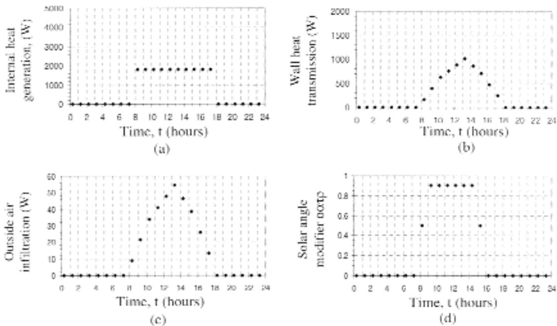
Figure 7: Hourly input values of the internal heat generation (a), heat transmission through the walls (b) outside air heat infiltration (c) and solar radiation incidence angle modifier (d)
