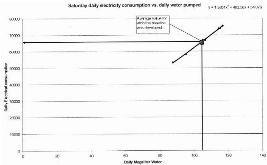
Figure 7: Daily water pumped and electricity consumption scatter plot
