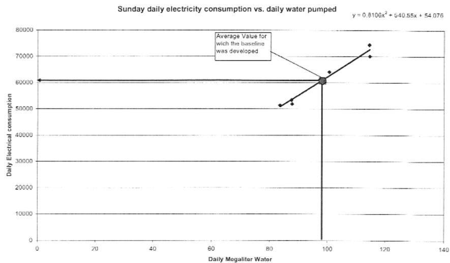
Figure 9: Daily water pumped and electricity consumption plot
