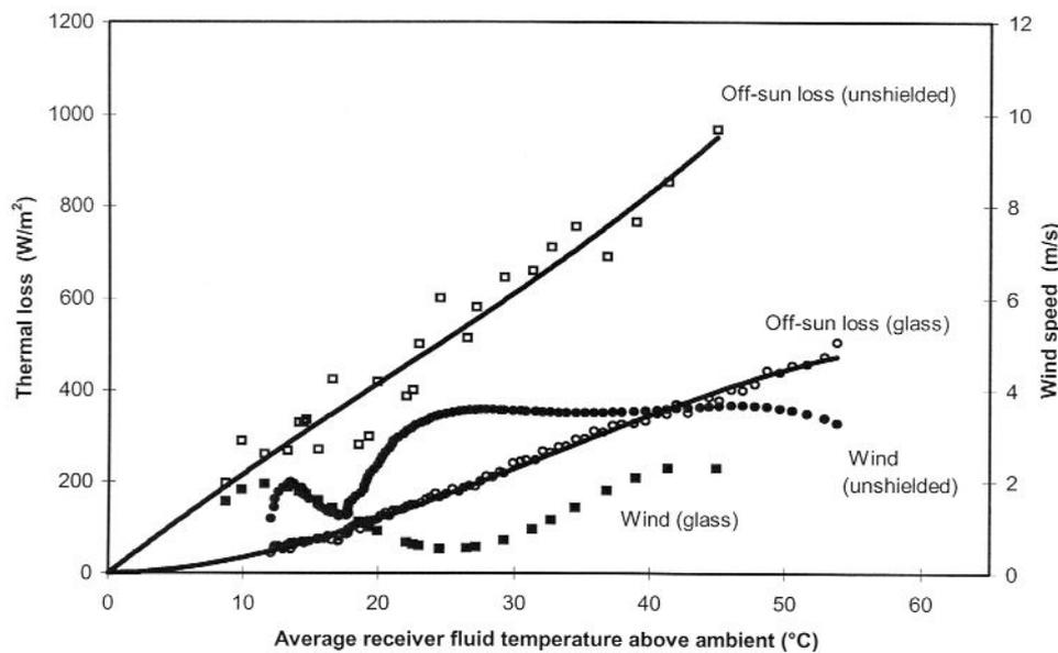
Figure 11: Thermal loss results for both receiver types
