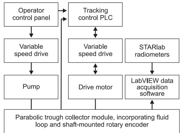
**Figure 1: Information flow between components of the PTSC test system**
