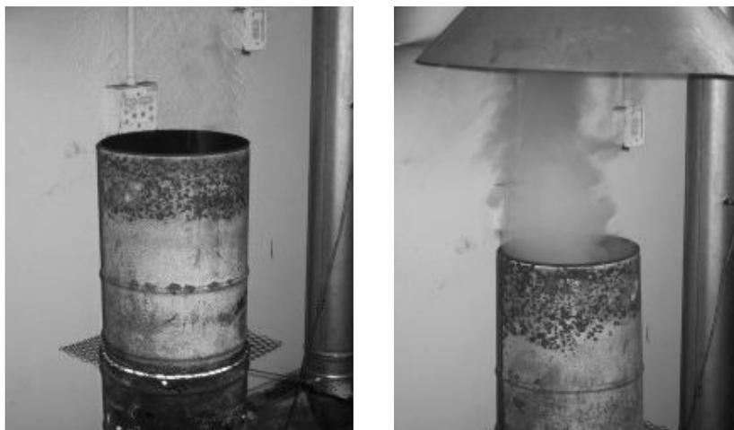
**Figure 1: Comparative smoke emissions from the Basa Magogo fire (left) and the fire ignited with the bottoms-up method (right)**
