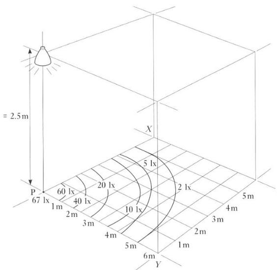
**Figure 2: An Isolux diagram**
