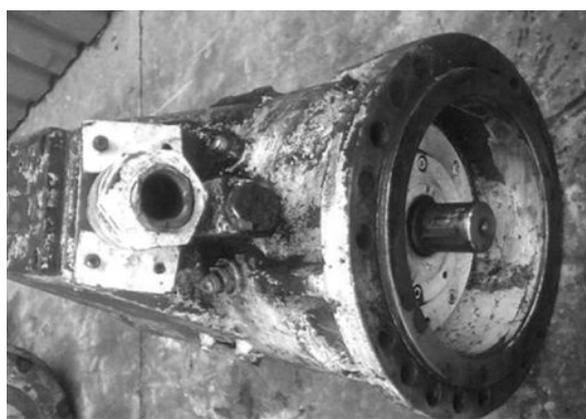
**Photo 4: Gathering arm (spinner) motor fitted with MCFR, after 1.8 years working underground**
