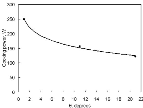
**Figure 6: Average cooking power as a function of incidence angle for water-based tests (Brooks, 2006)**
