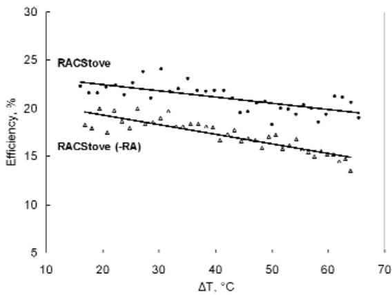
**Figure 4: Effect of the ring array concentrator on thermal efficiency in the standard testing range with water as the working fluid**
