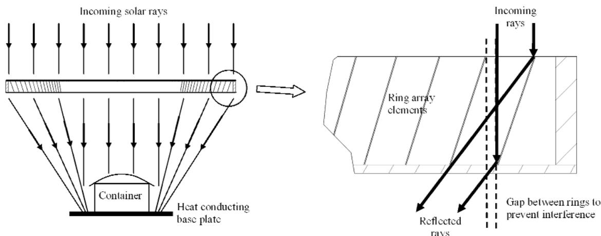
**Figure 1: Schematic of RACStove operation for a horizontally-aligned ring array with concentrated sunlight focused on oven base plate (left), and detail of reflected solar ray path between mirror elements (right)**
