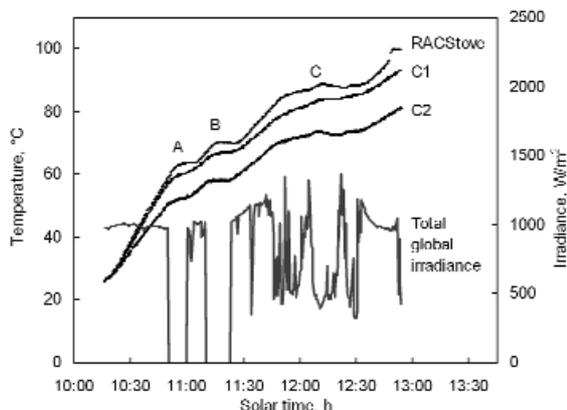
**Figure 12: Comparative oven performance under a typical duty cycle comprising two periods of complete shading lasting 10 minutes and 13 minutes (A and B respectively) and an extended period of non-tracking combined with variable irradiance lasting 40 minutes (C)**
