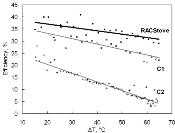
**Figure 8: Efficiency for near-normal incidence conditions with tracking and averaged irradiance  $G_{DN} = 903 \text{ W/m}^2$**
