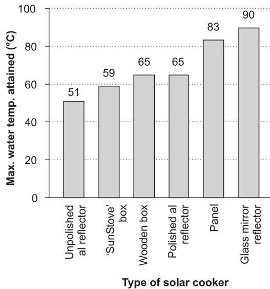
**Figure 3: Maximum water temperature attained**
