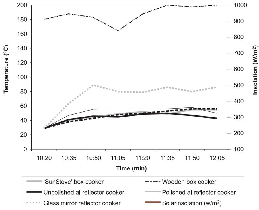
Figure 1: Water temperature variations and insolation against time on a sunny day
