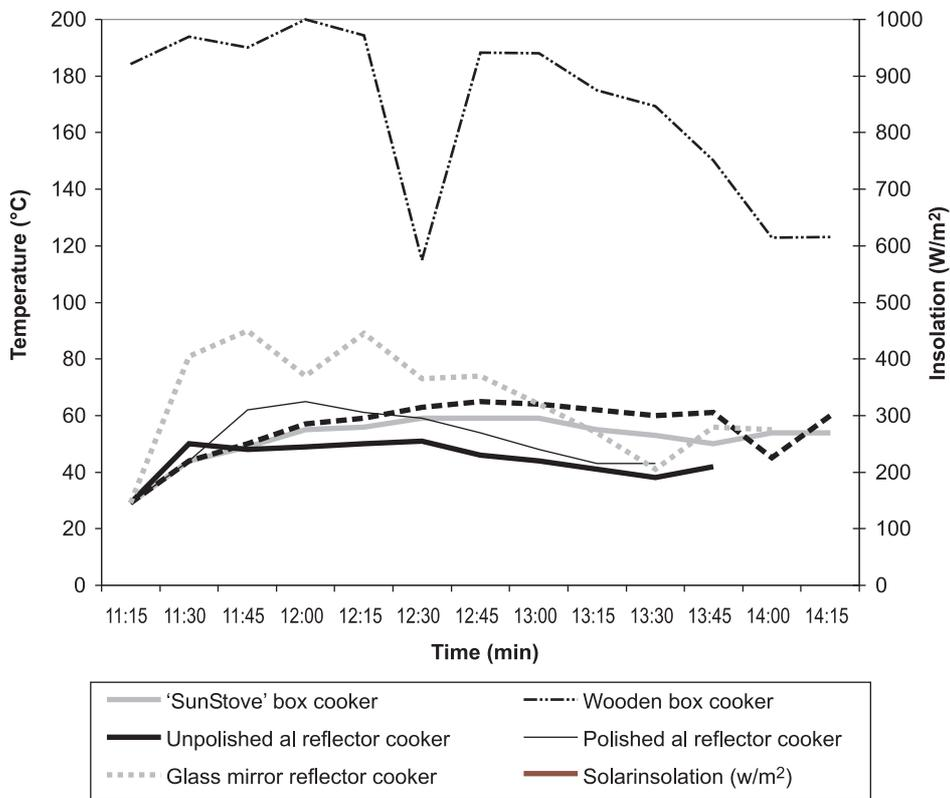
Figure 2: Water temperature variations and insolation against time on a cloudy day
