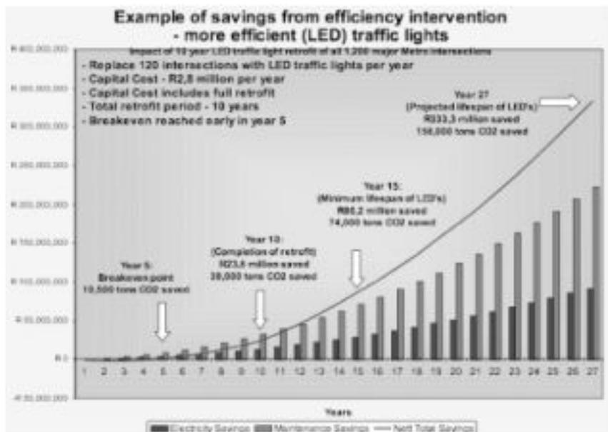
**Figure 1: Projected cumulative savings of maintenance and electricity consumption over 27 years based on the use of the retrofitted LED traffic signals in Cape Town**
