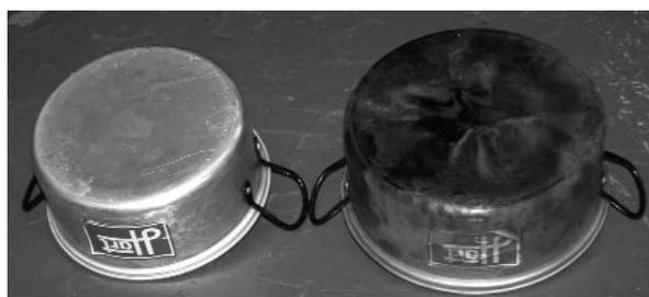
**Figure 7: Pot on right blackened after boiling water once using ethanol fuel in a prototype cooker**
