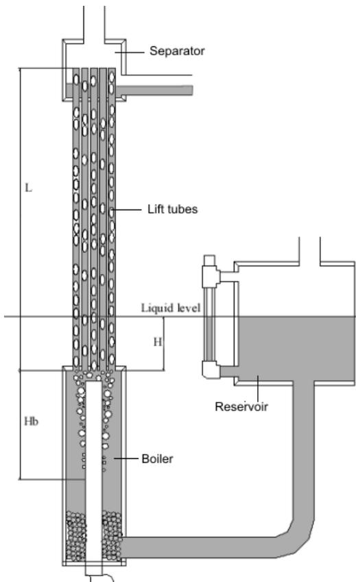
$L = 445 \text{ mm}$ ,  $H = 65 \text{ mm}$   $H_b = \text{approximately } 100 \text{ mm}$ , lift tube diameter =  $0.006 \text{ m}$ , heating element  $20 \text{ mm}$  and boiler diameter  $65 \text{ mm}$
