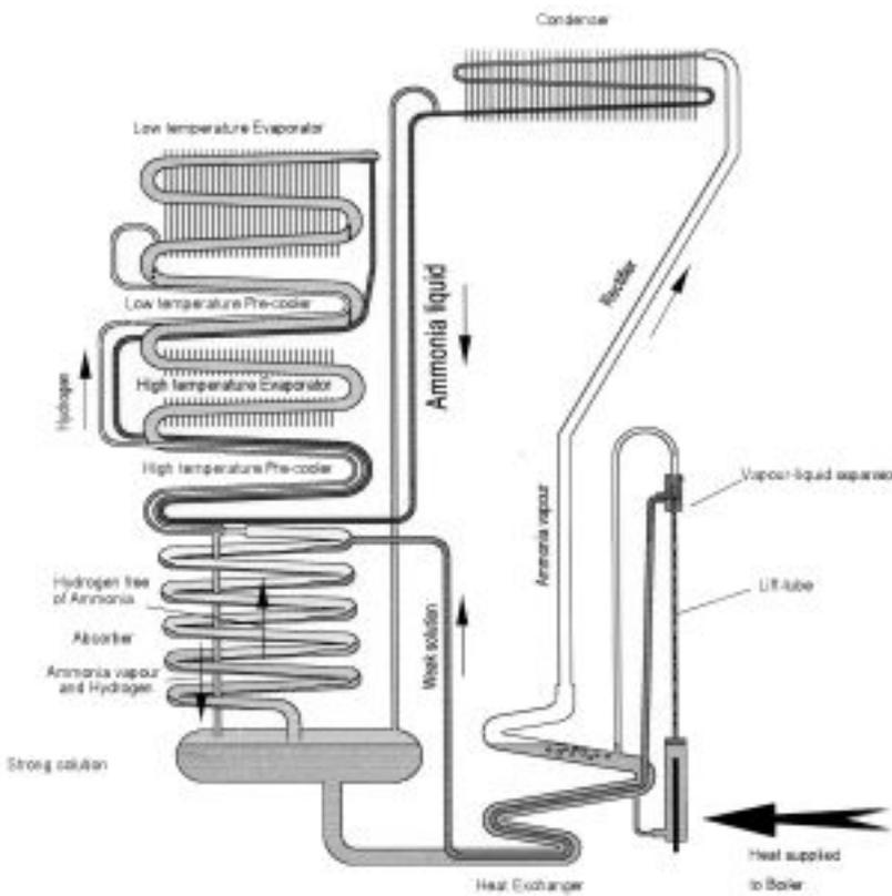
Figure 1: Diagram of a diffusion absorption refrigerator
