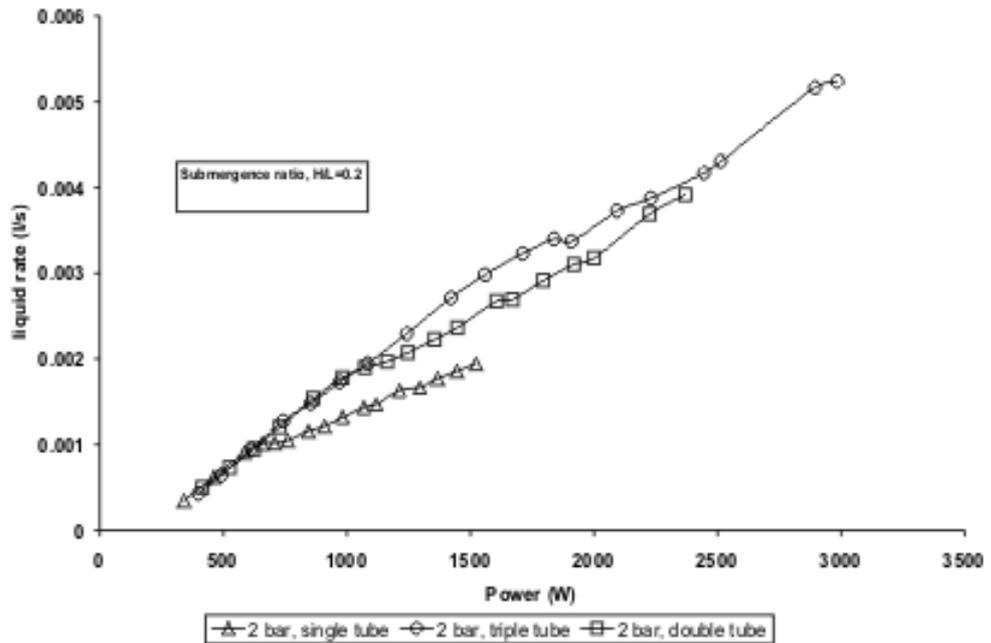
Figure 4 (first part): Comparison of tube configuration for 0, 2, 4 and 6 bar pressures
