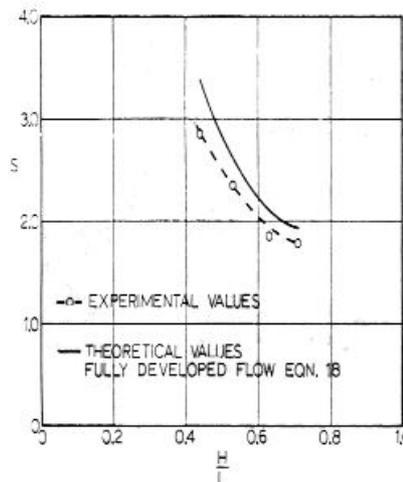
**Figure 5: Graph of Slip values for specific submergence ratio values 's'**
