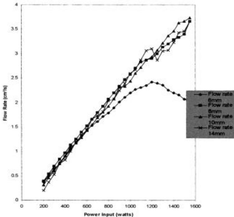
Figure 2: Characteristics of a single lift tube bubble pump
