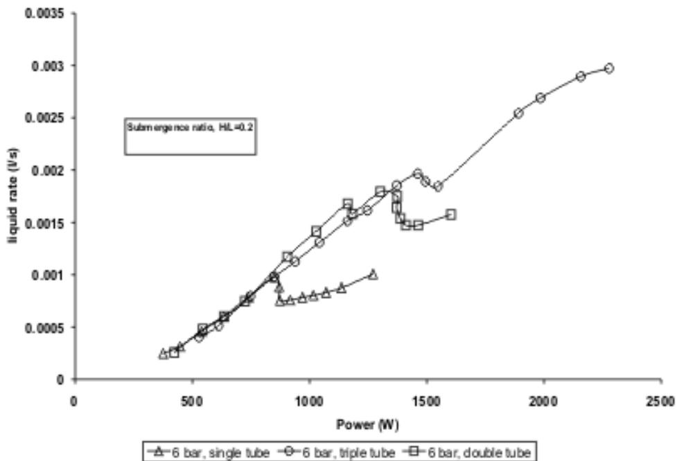
Figure 4 (continued): Comparison of tube configuration for 0, 2, 4 and 6 bar pressures
