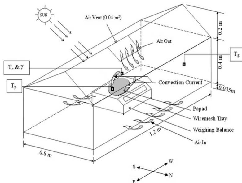
Figure 1: Schematic view of the experimental unit
