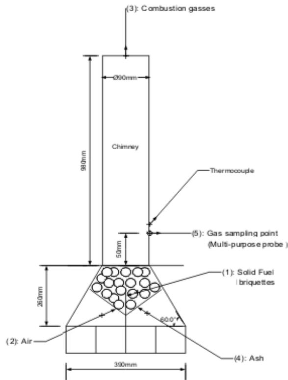
**Figure 2: Schematic diagram of the combustion system used**
