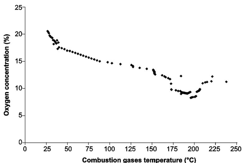
**Figure 3: Flue gas temperatures with oxygen concentrations**
